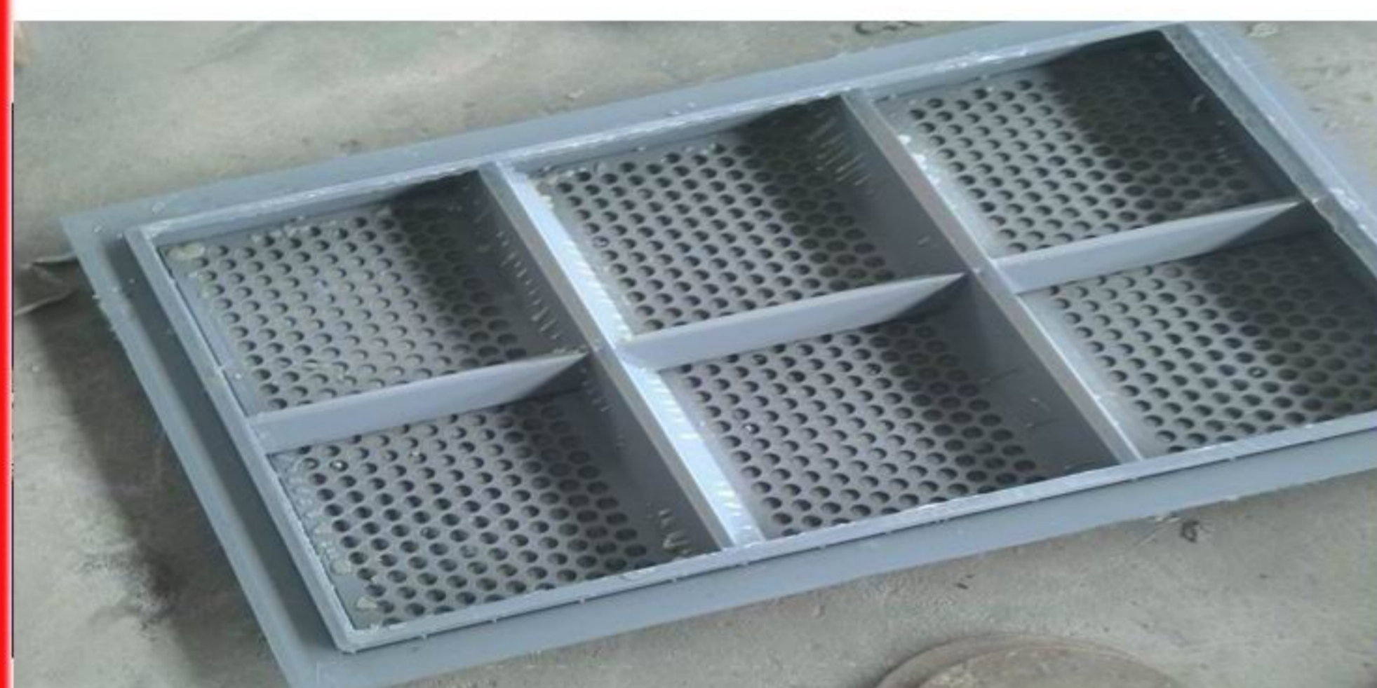
Support deck frame
