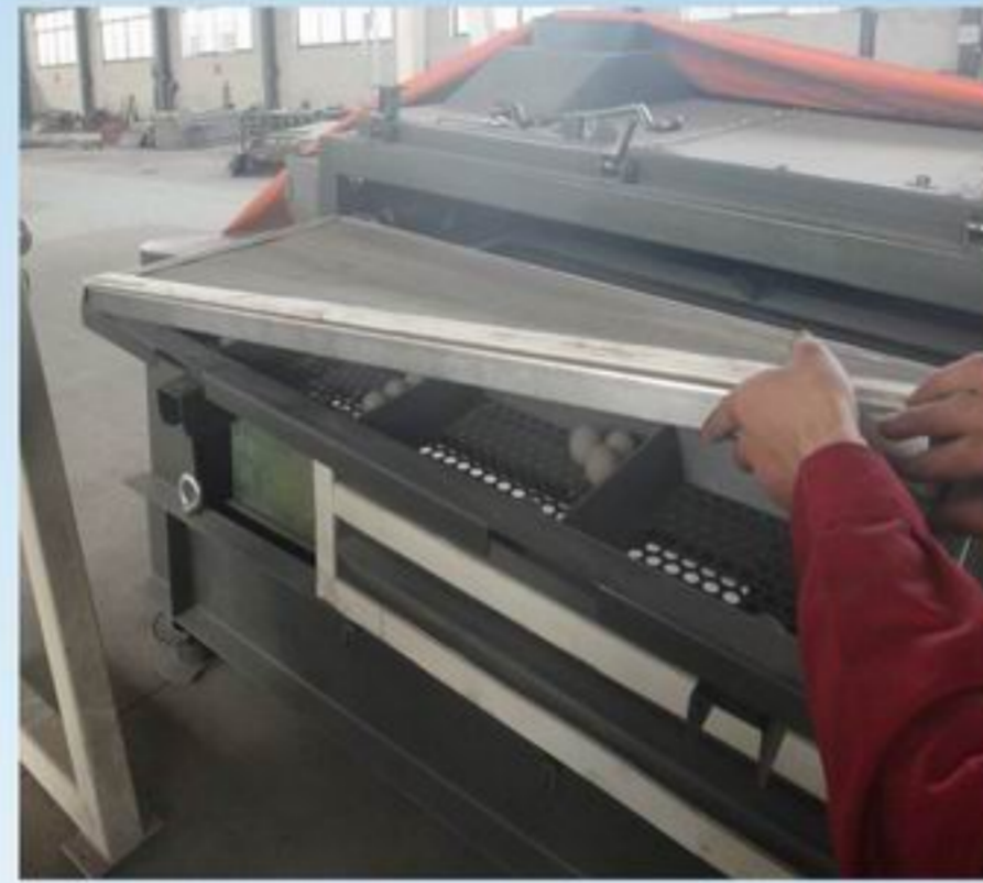
One operator could finish the mesh changing work, it is safe and save labor.
