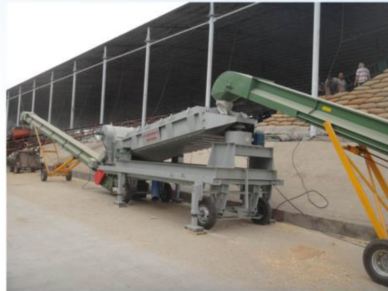
Screener MH-TC24 (bottom) For Screening PVC pellets at site
