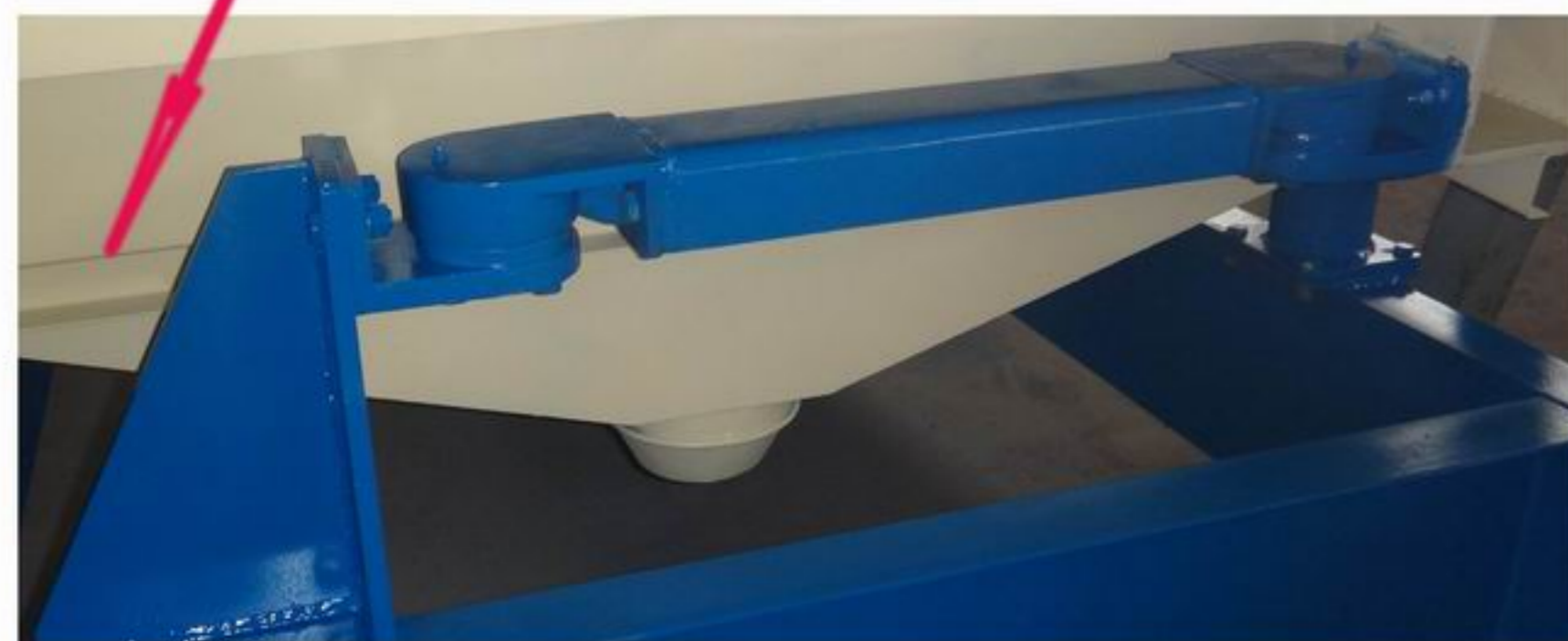
The guid bar on the material discharge end
